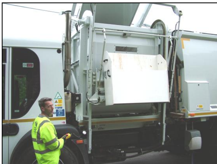
Below: Food waste is deposited in a separate compartment using a hydraulic system on the new lorries.
